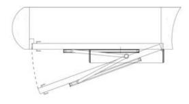
Push Arm Installation: Suitable for door wing opening outward (drive system inside)
